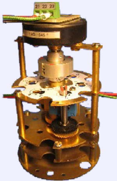
Precision Rotary Potentiometer mounted with Slip Clutch on Mechanical Limit Switch Set
